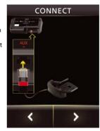
6. In the (second) CONNECT screen, shown left, connect the control cable attached to the GN1000 to the base's AUX port.
